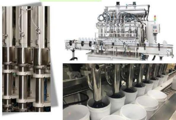
**Overflow Filling Machines:** Designed for cosmetic appeal, overflow fillers ensure that every container is filled to the same visual level, which is critical for products sold in transparent packaging. Specialized nozzles create a seal over the container opening and fill until the liquid reaches an overflow port. Any excess product is returned to the supply tank, guaranteeing a uniform appearance, making this method especially effective for managing foaming liquids.
